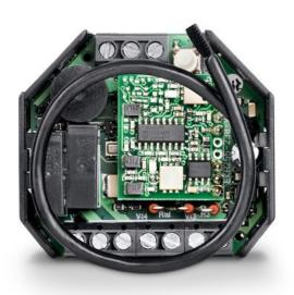
Receiving module for activating window drives with 230 V  $\,$  DC
